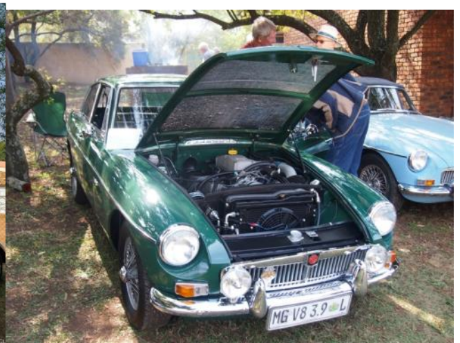
Hasia Botha's MGB GT V8 conversion, fitted with fuel injected 3.9L V8 with air-conditioning.
